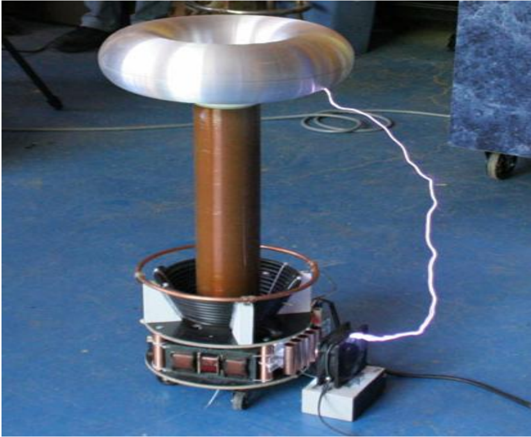
FIG 3 Tesla coil with rf current shorting to ground
